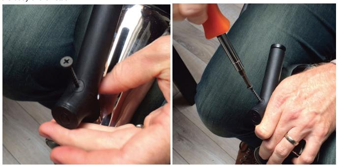
Start the threads and pull out the plug which will reveal the screw holding on the handle.
